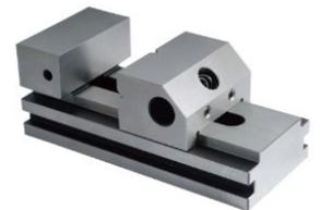
The third design has slots on both ends and both sides and is the only one I'd choose for a small mill. This allows alignment to either X or Y axes and a broad range of angles in between. With narrow clamps, it can also be mounted on its end or either side making it about as flexible as possible. Oddly enough, in spite of its superiority, it seems to be the most difficult to find. But they're out there and well worth the search.
